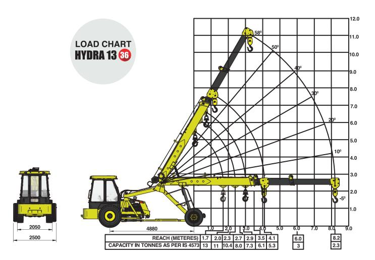
Rated loads are calculated for operation on leveled surface.
