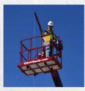
**Stow & Go Jib Winch** Stows in platform and requires no assembly. 500 lb. capacity in all positions eliminates guesswork.
