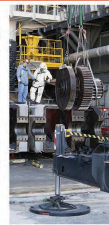
Crush Rating - The maximum allowable pressure. Working Load Limit - The maximum allowable load based on the application.
