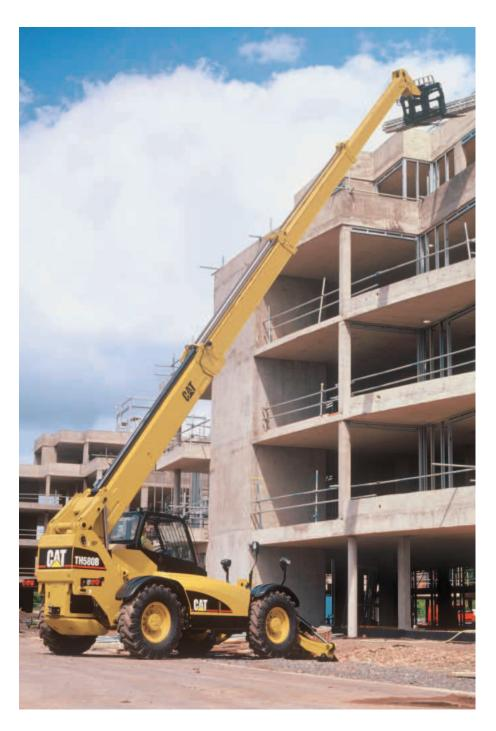
**Lift Height.** The TH580B can effectively and quickly place bricks, roofing materials and trusses to a maximum height of 17 m (56 ft).
