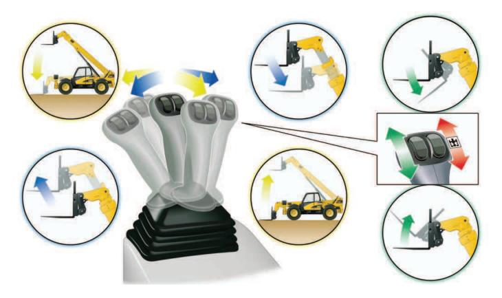
**Joystick Control.** The joystick allows three simultaneous boom functions and incorporates unique slider switches.
