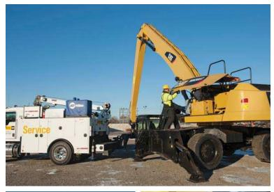
Primary service points are easily accessible through convenient panels and platforms on the sides and top of the machine. Components can be easily located with the engine and cooling system's longitudinal layout. Panels are hinged with gas struts, ensuring that one technician can easily access all maintenance points.
