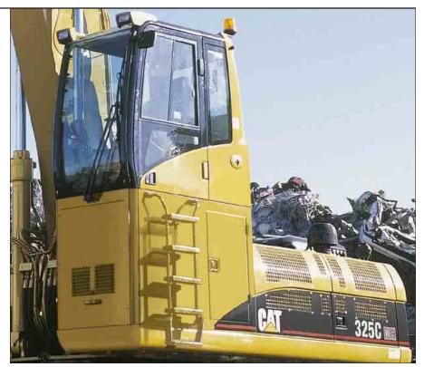
**Raised Cab.** The 1200 mm or 1600 mm raised cab further improves operator's visibility in all material handling applications. To reduce vibrations and sound the cab shell is attached to the frame with viscous mounts.
