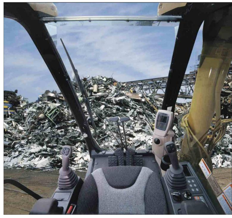
**Interior Operator Station.** The 325C MH operator work station is quiet with ergonomic control placement and convenient adjustments, low lever and pedal effort, ergonomic seat design and highly efficient ventilation.
