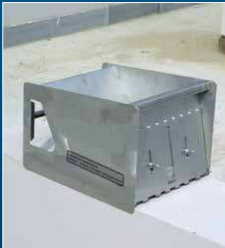
Mortar slides for all common brick types
