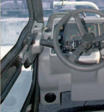
Two outer rear-view mirrors are fitted as standard, throughout the range. The cabin Bobcat® telescopic handlers rests on 3"Silentbloc" shock absorbers and is fitted to the chassis via the patented "Zebullon" suspension system, which absorbs impact energy when operating the telescopic handler.
