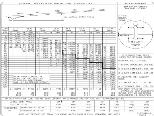
Note 1: When jib is erected, boom must be fully retracted before lowering below minimum boom with jib angles. Retracted boom with jib has no lifting capacity below a 50 degree angle with full span outriggers and below a 65 degree angle not shown on jib load rating chart.
