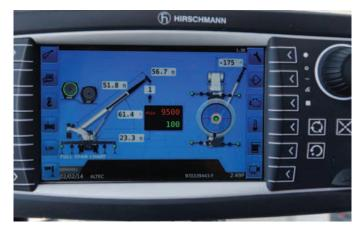
The convenient LMAP menu navigation with an intuitive user interface displays load on hook, rated capacity percentage, boom length and angle, load radius, and operator-defined protection with audible alarms. While the intuitive display and user interface are unique to Altec, the system's hardware consists of common "off-the-shelf" components that were critically selected for their performance and serviceability.
