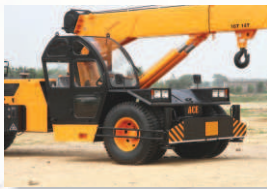
1 CABIN Front mounted, ergonomically designed spacious Cabin for better visibility & driveability.
